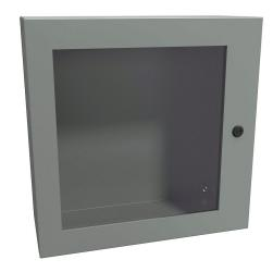
Hammond Eclipse series enclosure, NEMA 3R/4/12,  $20 \times 20 \times 8in$  (HxWxD), wall mount, carbon steel, ANSI 61 gray, powder coat finish, single-door, 1/4-turn semi-flush latch, polycarbonate window.
