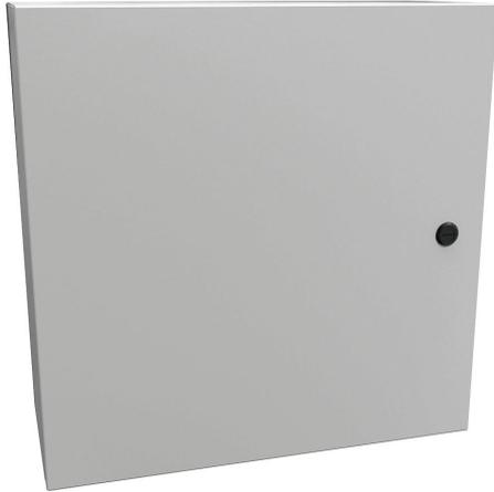
Hammond Eclipse series enclosure, NEMA 3R/4/12, 20 x 20 x 8in (HxWxD), wall mount, carbon steel, RAL 7035 light gray, powder coat finish, single-door, 1/4-turn semi-flush latch.
