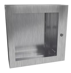
Hammond Eclipse series enclosure, NEMA 3R/4/4X/12/13,  $20 \times 20 \times 6$  in (HxWxD), wall mount, 304 stainless steel, #4 brush finish, single-door, 1/4-turn semi-flush 316 stainless steel latch, polycarbonate window.
