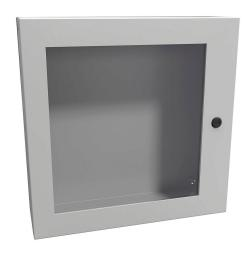
Hammond Eclipse series enclosure, NEMA 3R/4/12,  $20 \times 20 \times 6$ in (HxWxD), wall mount, carbon steel, RAL 7035 light gray, powder coat finish, single-door, 1/4-turn semi-flush latch, polycarbonate window.
