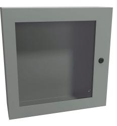
Hammond Eclipse series enclosure, NEMA 3R/4/12, 20 x 20 x 6in (HxWxD), wall mount, carbon steel, ANSI 61 gray, powder coat finish, single-door, 1/4-turn semi-flush latch, polycarbonate window.
