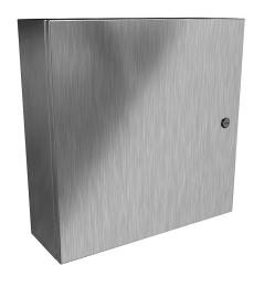
Hammond Eclipse series enclosure, NEMA 3R/4/4X/12/13, 20 x 20 x 6in (HxWxD), wall mount, 304 stainless steel, #4 brush finish, single-door, 1/4-turn semi-flush 316 stainless steel latch.
