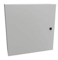
Hammond Eclipse series enclosure, NEMA 3R/4/12,  $20 \times 20 \times 6in$  (HxWxD), wall mount, carbon steel, RAL 7035 light gray, powder coat finish, single-door, 1/4-turn semi-flush latch.
