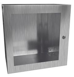
Hammond Eclipse series enclosure, NEMA 3R/4/4X/12/13, 20 x 20 x 12in (HxWxD), wall mount, 304 stainless steel, #4 brush finish, single-door, 1/4-turn semi-flush 316 stainless steel latch, polycarbonate window.
