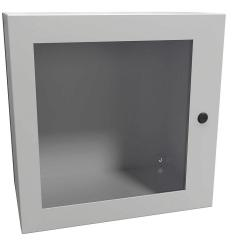
Hammond Eclipse series enclosure, NEMA 3R/4/12, 20 x 20 x 12in (HxWxD), wall mount, carbon steel, RAL 7035 light gray, powder coat finish, single-door, 1/4-turn semi-flush latch, polycarbonate window.
