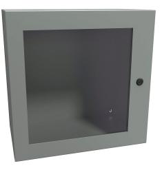
Hammond Eclipse series enclosure, NEMA 3R/4/12, 20 x 20 x 12in (HxWxD), wall mount, carbon steel, ANSI 61 gray, powder coat finish, single-door, 1/4-turn semi-flush latch, polycarbonate window.
