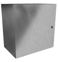
Hammond Eclipse series enclosure, NEMA 3R/4/4X/12/13, 20 x 20 x 12in (HxWxD), wall mount, 304 stainless steel, #4 brush finish, single-door, 1/4-turn semi-flush 316 stainless steel latch.
