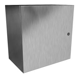
Hammond Eclipse series enclosure, NEMA 3R/4/4X/12/13,  $20 \times 20 \times 12$ in (HxWxD), wall mount, 316 stainless steel, #4 brush finish, single-door, 1/4-turn semi-flush 316 stainless steel latch.
