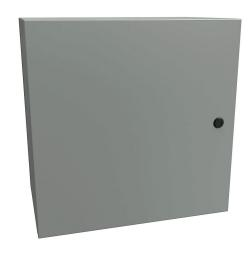
Hammond Eclipse series enclosure, NEMA 3R/4/12, 20 x 20 x 12in (HxWxD), wall mount, carbon steel, ANSI 61 gray, powder coat finish, single-door, 1/4-turn semi-flush latch.
