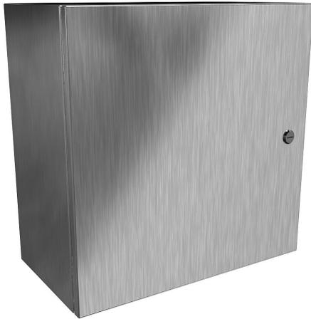
Hammond Eclipse series enclosure, NEMA 3R/4/4X/12/13, 20 x 20 x 10in (HxWxD), wall mount, 304 stainless steel, #4 brush finish, single-door, 1/4-turn semi-flush 316 stainless steel latch.
