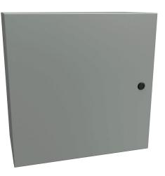
Hammond Eclipse series enclosure, NEMA 3R/4/12, 20 x 20 x 10in (HxWxD), wall mount, carbon steel, ANSI 61 gray, powder coat finish, single-door, 1/4-turn semi-flush latch.
