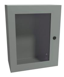
Hammond Eclipse series enclosure, NEMA 3R/4/12,  $20 \times 16 \times 8$ in (HxWxD), wall mount, carbon steel, ANSI 61 gray, powder coat finish, single-door, 1/4-turn semi-flush latch, polycarbonate window.
