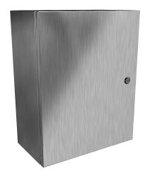
Hammond Eclipse series enclosure, NEMA 3R/4/4X/12/13, 20 x 16 x 8in (HxWxD), wall mount, 304 stainless steel, #4 brush finish, single-door, 1/4-turn semi-flush 316 stainless steel latch.
