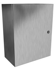
Hammond Eclipse series enclosure, NEMA 3R/4/4X/12/13, 20 x 16 x 8in (HxWxD), wall mount, 316 stainless steel, #4 brush finish, single-door, 1/4-turn semi-flush 316 stainless steel latch.
