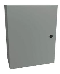
Hammond Eclipse series enclosure, NEMA 3R/4/12,  $20 \times 16 \times 8in$  (HxWxD), wall mount, carbon steel, ANSI 61 gray, powder coat finish, single-door, 1/4-turn semi-flush latch.
