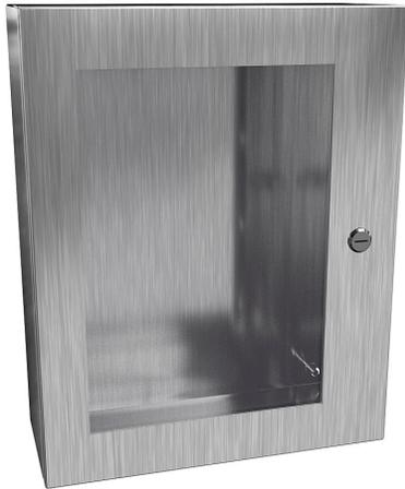
Hammond Eclipse series enclosure, NEMA 3R/4/4X/12/13, 20 x 16 x 6in (HxWxD), wall mount, 304 stainless steel, #4 brush finish, single-door, 1/4-turn semi-flush 316 stainless steel latch, polycarbonate window.
