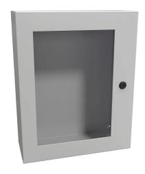
Hammond Eclipse series enclosure, NEMA 3R/4/12,  $20 \times 16 \times 6$  in (HxWxD), wall mount, carbon steel, RAL 7035 light gray, powder coat finish, single-door, 1/4-turn semi-flush latch, polycarbonate window.
