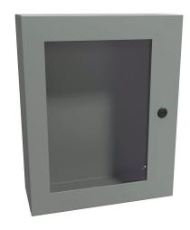
Hammond Eclipse series enclosure, NEMA 3R/4/12,  $20 \times 16 \times 6$  in (HxWxD), wall mount, carbon steel, ANSI 61 gray, powder coat finish, single-door, 1/4-turn semi-flush latch, polycarbonate window.
