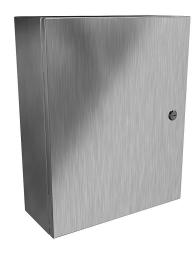
Hammond Eclipse series enclosure, NEMA 3R/4/4X/12/13, 20 x 16 x 6in (HxWxD), wall mount, 304 stainless steel, #4 brush finish, single-door, 1/4-turn semi-flush 316 stainless steel latch.
