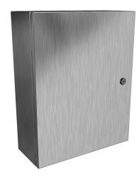
Hammond Eclipse series enclosure, NEMA 3R/4/4X/12/13, 20 x 16 x 6in (HxWxD), wall mount, 316 stainless steel, #4 brush finish, single-door, 1/4-turn semi-flush 316 stainless steel latch.
