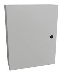
Hammond Eclipse series enclosure, NEMA 3R/4/12,  $20 \times 16 \times 6$ in (HxWxD), wall mount, carbon steel, RAL 7035 light gray, powder coat finish, single-door, 1/4-turn semi-flush latch.
