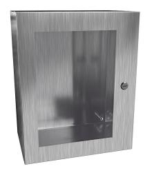
Hammond Eclipse series enclosure, NEMA 3R/4/4X/12/13,  $20 \times 16 \times 10$  in (HxWxD), wall mount, 304 stainless steel, #4 brush finish, single-door, 1/4-turn semi-flush 316 stainless steel latch, polycarbonate window.
