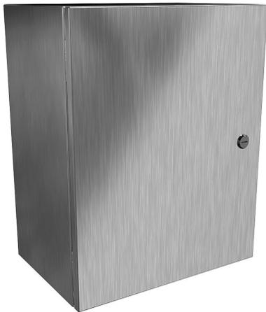
Hammond Eclipse series enclosure, NEMA 3R/4/4X/12/13, 20 x 16 x 10in (HxWxD), wall mount, 304 stainless steel, #4 brush finish, single-door, 1/4-turn semi-flush 316 stainless steel latch.
