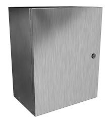
Hammond Eclipse series enclosure, NEMA 3R/4/4X/12/13, 20 x 16 x 10in (HxWxD), wall mount, 316 stainless steel, #4 brush finish, single-door, 1/4-turn semi-flush 316 stainless steel latch.
