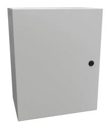
Hammond Eclipse series enclosure, NEMA 3R/4/12, 20 x 16 x 10in (HxWxD), wall mount, carbon steel, RAL 7035 light gray, powder coat finish, single-door, 1/4-turn semi-flush latch.
