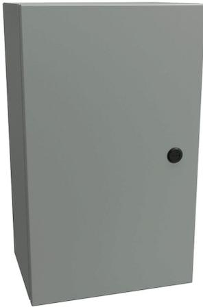
Hammond Eclipse series enclosure, NEMA 3R/4/12, 20 x 12 x 8in (HxWxD), wall mount, carbon steel, ANSI 61 gray, powder coat finish, single-door, 1/4-turn semi-flush latch.
