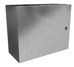
Hammond Eclipse series enclosure, NEMA 3R/4/4X/12/13,  $16 \times 20 \times 8$  in (HxWxD), wall mount, 316 stainless steel, #4 brush finish, single-door, 1/4-turn semi-flush 316 stainless steel latch.
