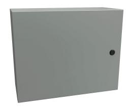
Hammond Eclipse series enclosure, NEMA 3R/4/12,  $16 \times 20 \times 8in$  (HxWxD), wall mount, carbon steel, ANSI 61 gray, powder coat finish, single-door, 1/4-turn semi-flush latch.
