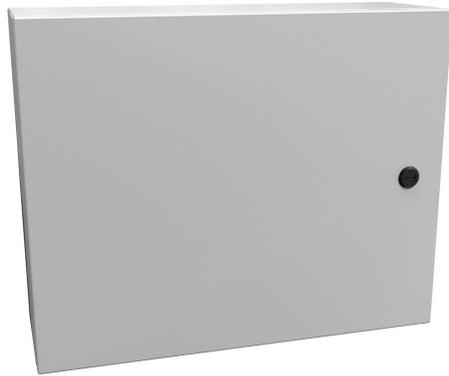
Hammond Eclipse series enclosure, NEMA 3R/4/12, 16 x 20 x 6in (HxWxD), wall mount, carbon steel, RAL 7035 light gray, powder coat finish, single-door, 1/4-turn semi-flush latch.
