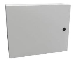
Hammond Eclipse series enclosure, NEMA 3R/4/12,  $16 \times 20 \times 6$ in (HxWxD), wall mount, carbon steel, RAL 7035 light gray, powder coat finish, single-door, 1/4-turn semi-flush latch.
