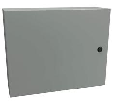
Hammond Eclipse series enclosure, NEMA 3R/4/12, 16 x 20 x 6in (HxWxD), wall mount, carbon steel, ANSI 61 gray, powder coat finish, single-door, 1/4-turn semi-flush latch.
