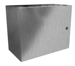
Hammond Eclipse series enclosure, NEMA 3R/4/4X/12/13,  $16 \times 20 \times 10$  in (HxWxD), wall mount, 304 stainless steel, #4 brush finish, single-door, 1/4-turn semi-flush 316 stainless steel latch.
