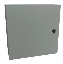
Hammond Eclipse series enclosure, NEMA 3R/4/12,  $16 \times 16 \times 8in$  (HxWxD), wall mount, carbon steel, ANSI 61 gray, powder coat finish, single-door, 1/4-turn semi-flush latch.
