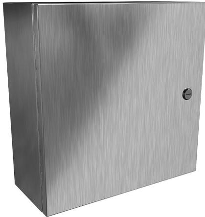
Hammond Eclipse series enclosure, NEMA 3R/4/4X/12/13, 16 x 16 x 6in (HxWxD), wall mount, 304 stainless steel, #4 brush finish, single-door, 1/4-turn semi-flush 316 stainless steel latch.
