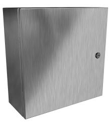
Hammond Eclipse series enclosure, NEMA 3R/4/4X/12/13, 16 x 16 x 6in (HxWxD), wall mount, 304 stainless steel, #4 brush finish, single-door, 1/4-turn semi-flush 316 stainless steel latch.
