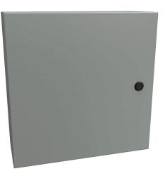
Hammond Eclipse series enclosure, NEMA 3R/4/12, 16 x 16 x 6in (HxWxD), wall mount, carbon steel, ANSI 61 gray, powder coat finish, single-door, 1/4-turn semi-flush latch.
