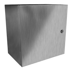
Hammond Eclipse series enclosure, NEMA 3R/4/4X/12/13,  $16 \times 10$  in (HxWxD), wall mount, 304 stainless steel, #4 brush finish, single-door, 1/4-turn semi-flush 316 stainless steel latch.
