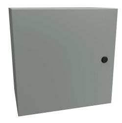
Hammond Eclipse series enclosure, NEMA 3R/4/12, 16 x 16 x 10in (HxWxD), wall mount, carbon steel, ANSI 61 gray, powder coat finish, single-door, 1/4-turn semi-flush latch.
