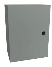
Hammond Eclipse series enclosure, NEMA 3R/4/12,  $16 \times 12 \times 8in$  (HxWxD), wall mount, carbon steel, ANSI 61 gray, powder coat finish, single-door, 1/4-turn semi-flush latch.
