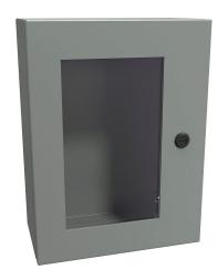
Hammond Eclipse series enclosure, NEMA 3R/4/12,  $16 \times 12 \times 6$ in (HxWxD), wall mount, carbon steel, ANSI 61 gray, powder coat finish, single-door, 1/4-turn semi-flush latch, polycarbonate window.
