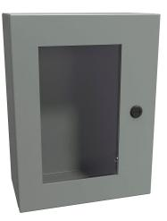
Hammond Eclipse series enclosure, NEMA 3R/4/12, 16 x 12 x 6in (HxWxD), wall mount, carbon steel, ANSI 61 gray, powder coat finish, single-door, 1/4-turn semi-flush latch, polycarbonate window.
