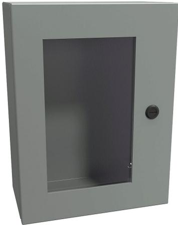
Hammond Eclipse series enclosure, NEMA 3R/4/12, 16 x 12 x 6in (HxWxD), wall mount, carbon steel, ANSI 61 gray, powder coat finish, single-door, 1/4-turn semi-flush latch, polycarbonate window.
