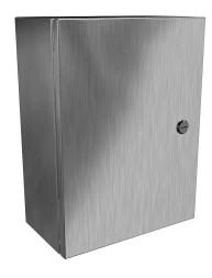
Hammond Eclipse series enclosure, NEMA 3R/4/4X/12/13, 16 x 12 x 6in (HxWxD), wall mount, 304 stainless steel, #4 brush finish, single-door, 1/4-turn semi-flush 316 stainless steel latch.
