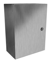
Hammond Eclipse series enclosure, NEMA 3R/4/4X/12/13, 16 x 12 x 6in (HxWxD), wall mount, 316 stainless steel, #4 brush finish, single-door, 1/4-turn semi-flush 316 stainless steel latch.
