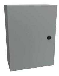
Hammond Eclipse series enclosure, NEMA 3R/4/12,  $16 \times 12 \times 6$ in (HxWxD), wall mount, carbon steel, ANSI 61 gray, powder coat finish, single-door, 1/4-turn semi-flush latch.
