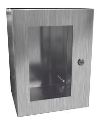
Hammond Eclipse series enclosure, NEMA 3R/4/4X/12/13,  $16 \times 12 \times 10$  in (HxWxD), wall mount, 304 stainless steel, #4 brush finish, single-door, 1/4-turn semi-flush 316 stainless steel latch, polycarbonate window.
