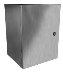
Hammond Eclipse series enclosure, NEMA 3R/4/4X/12/13,  $16 \times 12 \times 10$  in (HxWxD), wall mount, 304 stainless steel, #4 brush finish, single-door, 1/4-turn semi-flush 316 stainless steel latch.
