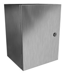
Hammond Eclipse series enclosure, NEMA 3R/4/4X/12/13,  $16 \times 12 \times 10$  in (HxWxD), wall mount, 316 stainless steel, #4 brush finish, single-door, 1/4-turn semi-flush 316 stainless steel latch.
