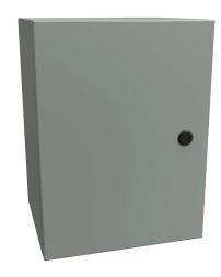
Hammond Eclipse series enclosure, NEMA 3R/4/12, 16 x 12 x 10in (HxWxD), wall mount, carbon steel, ANSI 61 gray, powder coat finish, single-door, 1/4-turn semi-flush latch.
