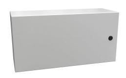
Hammond Eclipse series enclosure, NEMA 3R/4/12,  $12 \times 24 \times 8in$  (HxWxD), wall mount, carbon steel, RAL 7035 light gray, powder coat finish, single-door, 1/4-turn semi-flush latch.
